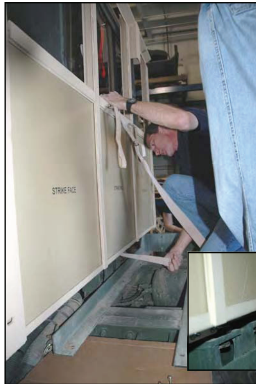
10) Guide long center strap behind the bottom center panel and loop through bottom hook and lock in place with attached buckle.
