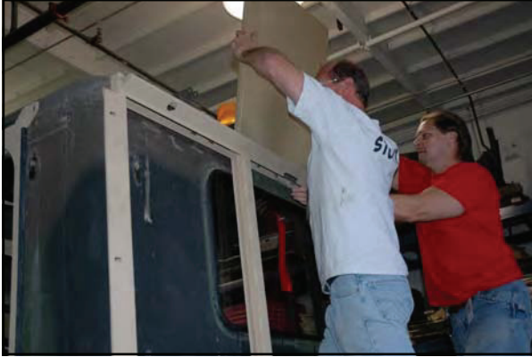
7.) Slide one armor panel in each of the three frame slots (this would equate to three panels across the bottom of the frame).
