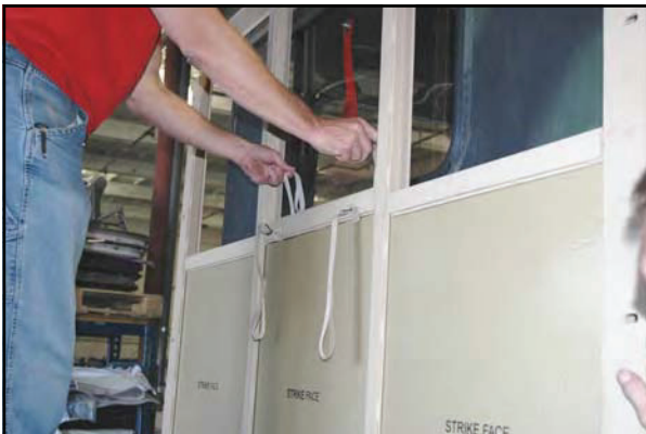
9.) Insert the three center support dividers across the rear cab bottom armor. (Ensure that on the middle bar the two straps facing the rear window are not tucked under but vertical against the rear window)
