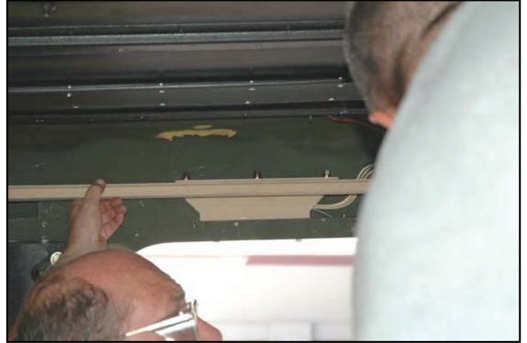
2.) Add washers and nuts to bolts on the door frame brackets and leave the middle bracket (located where the rear view mirror would be) for later installation.
