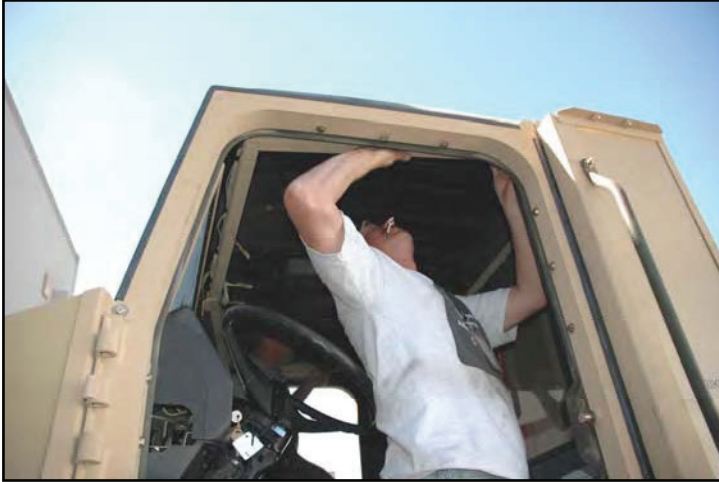
1.) Align roof frame with brackets installed earlier.
