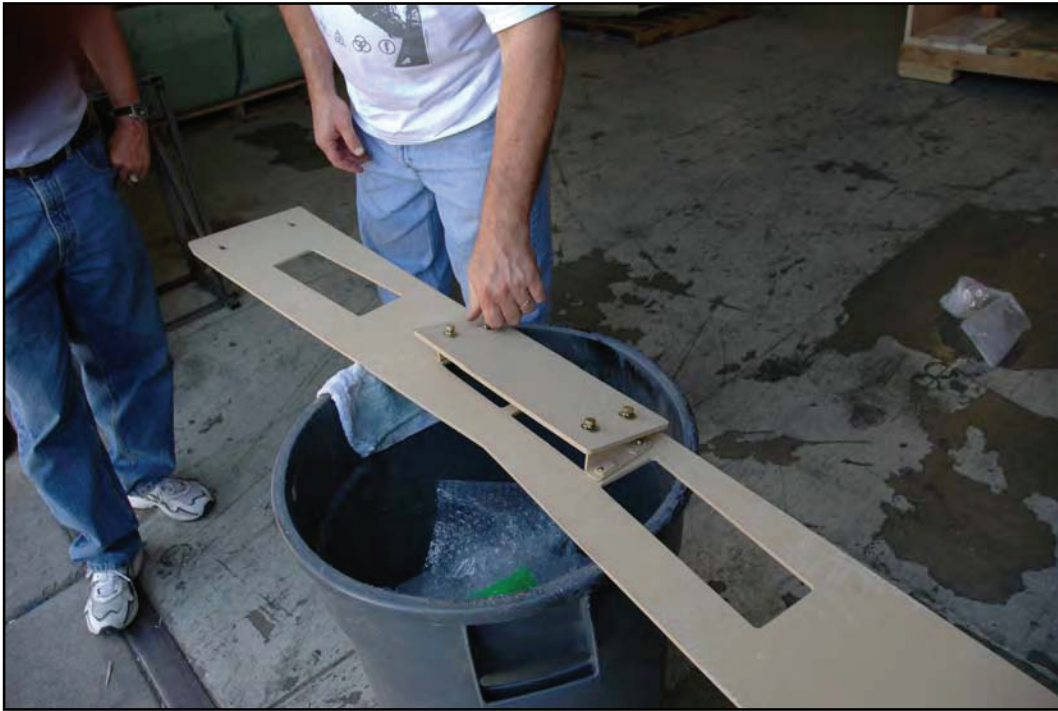
1.) Install nuts, bolts and washers on the intake cover.
