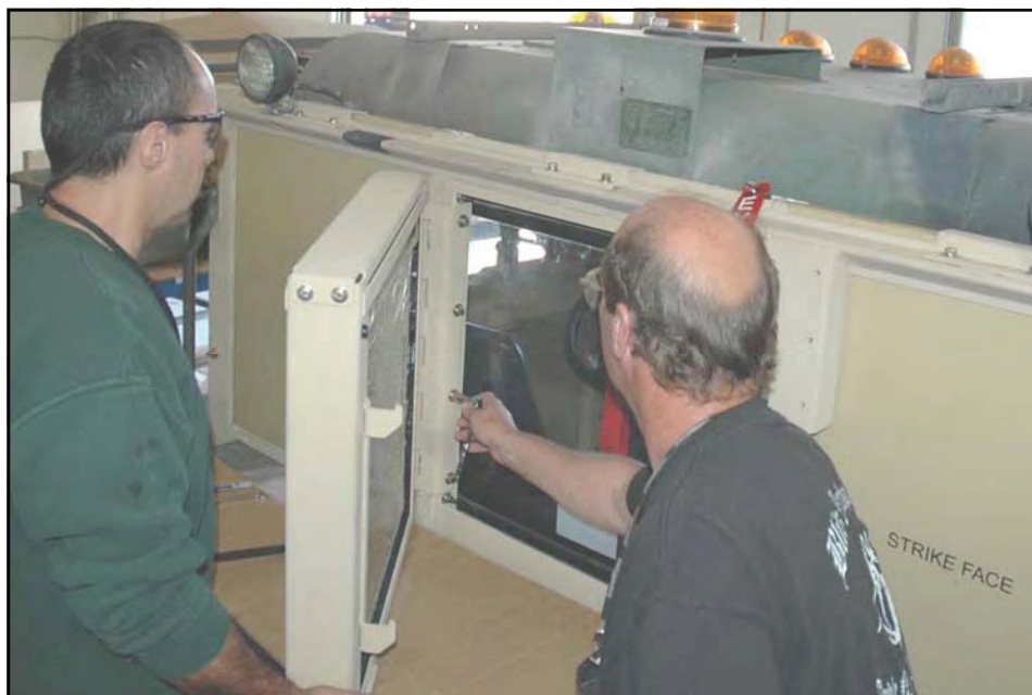
17. Install the Window Assembly using 5/16-18 x 3/4 bolts, flat washers and lock washers as shown.
